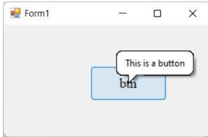
Fig: Tool Tip at work when Gotfocus event occurs
